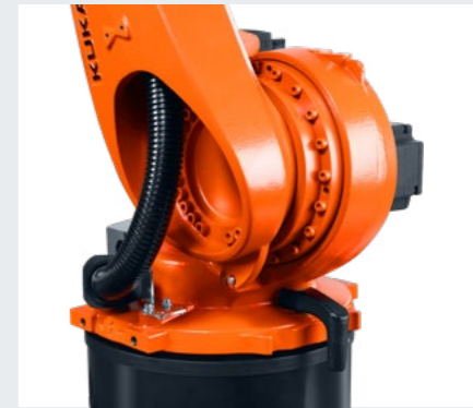
The space-saving and intelligently integrated cabling ensures that the KR CYBERTECH robots have maximum freedom of motion in any installation position.
