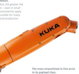
With an interference radius of just 67 mm, the KR CYBERTECH nano robots have the smallest in-line wrist in their class. Worldwide. It enables work to be carried out in positions that are inaccessible for other robots.
