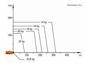
The KR 20 R3100 is designed for a rated payload of 20 kg in order to optimize the dynamic performance of the robot. With reduced load center distances, higher loads up to the maximum payload may be used. The specific load case must be verified using KUKA.Load. For further consultation, please contact KUKA Support.
